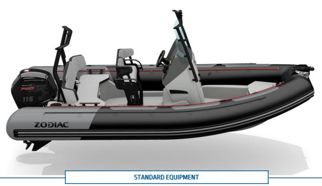
**HULL & DECK:** 1 Bow Bitt / 2 Aft Cleats , 1 Bow D Ring / 2 Towing Rings , 2 Bailers, Fairleads, GRP Deep V-Hull, Lockable Mooring Storage, Ski & Wakeboard Locker, Tilting Console.
