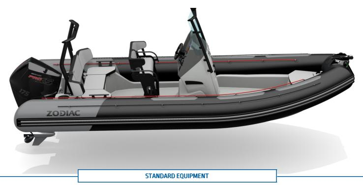
**HULL & DECK:** 1 Bow Bitt / 2 Aft Cleats , 1 Bow D Ring / 2 Towing Rings , 1 Mooring Kit [Mooring Chain + Anchor] , 2 Bailers, Fairleads, GRP Deep V-Hull, Lockable Mooring Storage , Self Bailing Countermoulded Deck [when empty] , Ski & Wakeboard Locker , Tilting Console.
